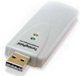
**Note** The effective range of most RF Receivers is about 200 feet (60 meters) and the Long Range Receiver is about 400 feet (120 meters). A single receiver is sufficient for up to 1000 ResponseCards, and a direct line of sight between the receiver and the ResponseCard is not necessary.
