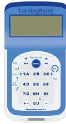
Responsive Innovations' ResponseCard XR—a compact response device that uses radio frequency technology to send audience responses and allows for self-paced testing by letting students enter responses to many different questions on the card's multi-line LCD; then transmitting all the answers at once.
